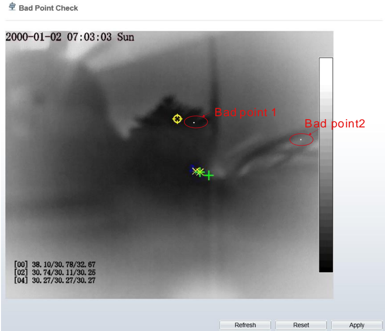
Figure 5-7 Bad Point Check
